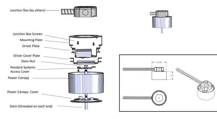
Powered Canopy Detail with Slope Ceiling Stem Mount Ordering Code: PRC-SLP - Powered Round Surface J-Box Canopy, Slope Ceiling
